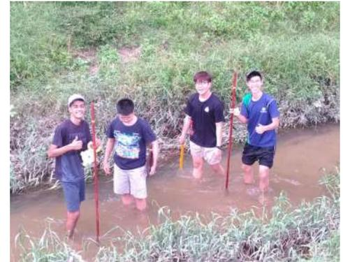
timed how long it took to go 10 metres and then calculated the speed of flow. Finally, they used two ranging poles and a clinometer on their phones to find the river channel's slope angle.
